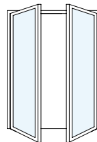
double leaf door outward opening w. 2000 | h. 2700 mm
